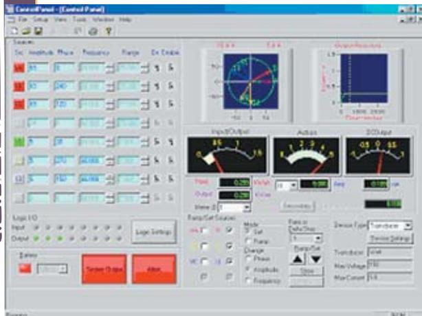
This graphical interface enables test engineers to quickly perform simple performance verification tests on all meters and transducers. It allows users to develop a library of automated tests based on their specific practices and test results.
